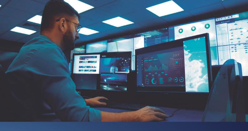
MultiVis Cockpit is an operator workspace that can act as a no-boundary network KVM, controlling up to eight remote terminals or virtual machines, regardless of the operating system. The client windows can be opened, positioned and resized as required. Simultaneous mouse and keyboard control allows the operator to smoothly change from one client desktop to another by simply moving the cursor through the windows.
