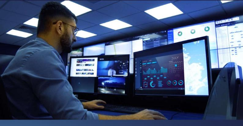
MultiVis Cockpit can act as a no-boundary network KVM, controlling up to eight remote terminals or virtual machines, no matter what the operating system. The desktop can be opened, positioned and resized as you see fit, with a simultaneous mouse and keyboard control the operator can smoothly change from one desktop to another by simply moving the cursor through the windows.
